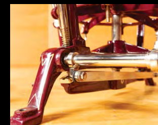
Full-length rocker arm and transfer bar for accurate pitch changes
